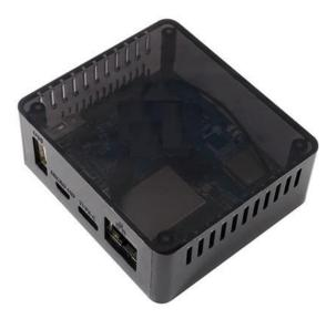
The HBI-VS is an IP intercom video server which supports camera monitoring for HomeScenario IP intercom indoor touch panels. The video streams can be taken from CCTV/ DVR, IP camera or NVR in the intranet. The indoor touch panels can select target camera channel and monitor the real-time video.
